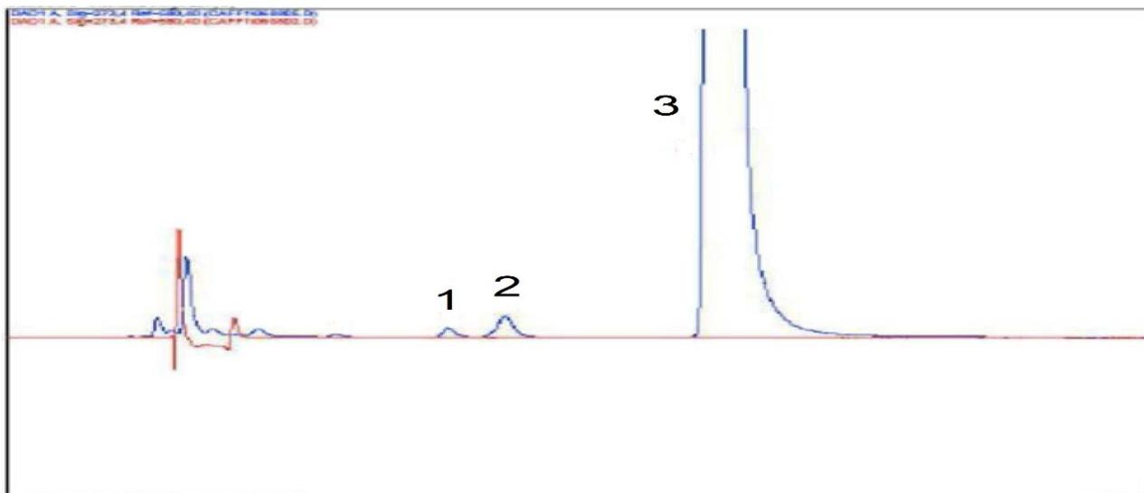
Fig. 2. A typical HPLC chromatogram shows the separation of caffeine (3) and paraxanthine (1). 7-[ $\beta$ -hydroxyethyl]theophylline (2) was used as an internal standard in caffeine biotransformation assay.
